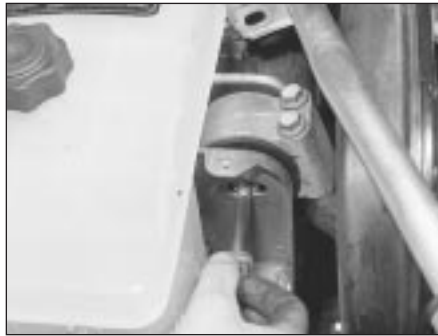
7.7 Undo the engine right-hand mounting through-bolt
