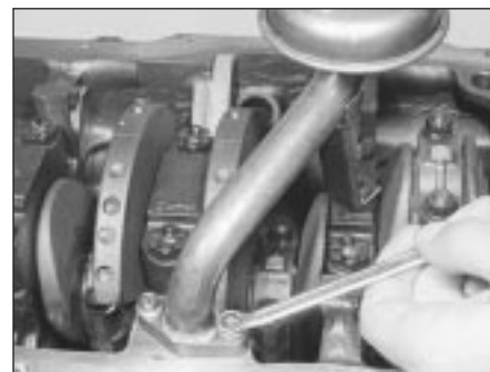
13.10 Undo the two pick-up pipe-to-crankcase bolts
