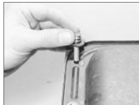
13.8 Sump special retaining bolt location
