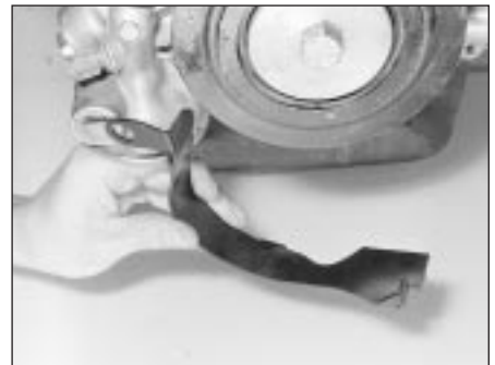
7.13 Removing the timing belt bottom cover
