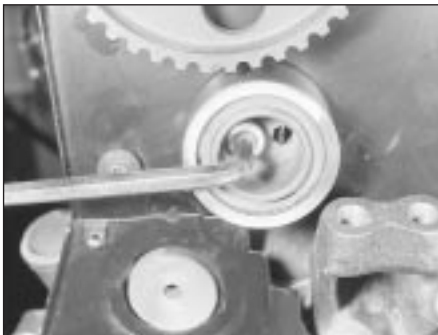
11.3 Undo the timing belt idler pulley bolt
